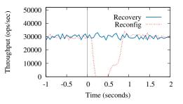
(a) Throughput during a single recovery and reconfiguration starting at time 0
