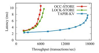
Fig. 16. Average Retwis transaction Latency (Zipf coefficient 0.75) versus throughput within a datacenter.
