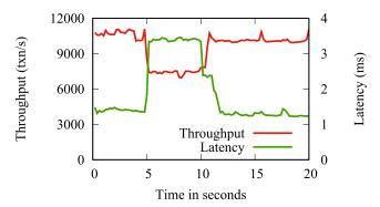
Fig. 20. Performance of TAPIR recovery protocol. One replica is failed at t = 5s, and restarted at t = 10s.
