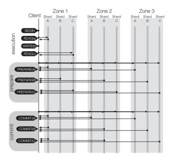
Fig. 6. *Example read-write transaction in TAPIR*. TAPIR executes the same transaction pictured in Figure 2 with less redundant coordination. Reads go to the closest replica and Prepare takes a single round-trip to all replicas in all shards. TAPIR sends Commit asynchronously, because participants will always come to the same commit decision (see Section 5.2.3). Overall, TAPIR is able to commit transactions in a single round-trip to all participating replicas.
