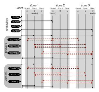
Fig. 2. Example read-write transaction using two-phase commit, viewstamped replication, and strict two-phase locking. Availability zones represent a cluster, datacenter, or geographic region. Each shard holds a partition of the data stored in the system and has replicas in each zone for fault tolerance. The red, dashed lines represent redundant coordination in the replication layer.
