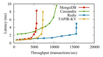
Fig. 19. Comparison with weakly consistent storage systems using the YCSB+T benchmark with one shard, three replicas, and 1M keys.
