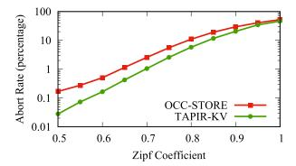
Fig. 18. Abort rates at varying Zipf co-efficients with a constant load of 5,000 transactions/second in a single datacenter. This graph excludes LOCK-STORE, which does not abort.
